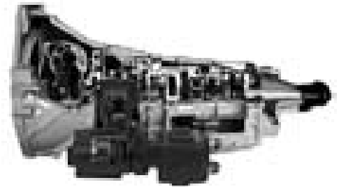
Transmission with PTO and hydraulic pump installed.
